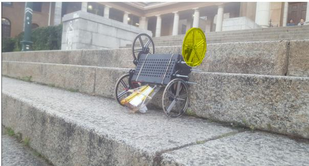
(c) step 3 of the desired motion for rotating the rear wheel on to the obstacle
