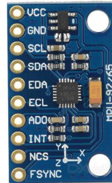
Figure 6.30: MPU-9255 9 degrees of freedom IC.
