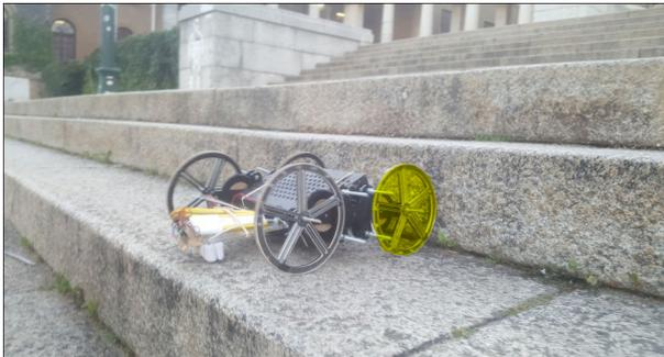
(a) step 1 of the desired motion for driving the front wheel on to the obstacle
