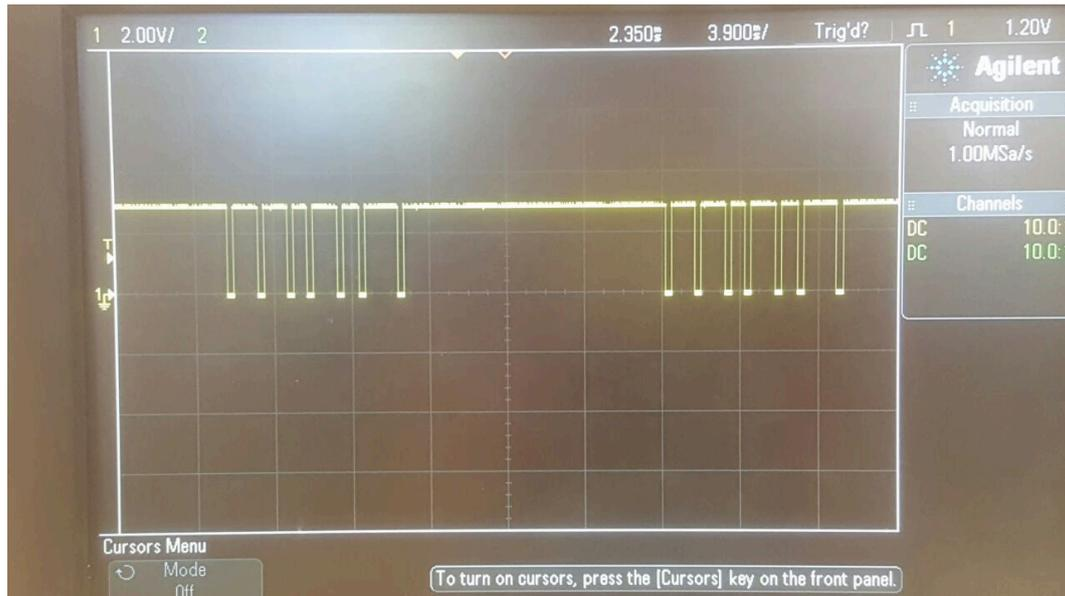
Figure 6.34: Normal waveform from RC receiver
