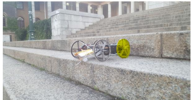
(f) step 6 of the desired motion for driving the front wheel on to the obstacle
