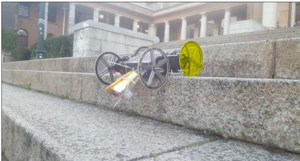
(e) step 5 of the desired motion for driving the front wheel on to the obstacle
