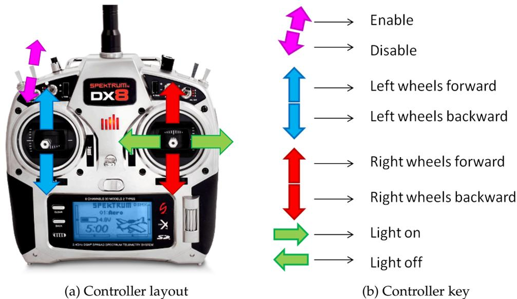
Figure 6.40: controller format
