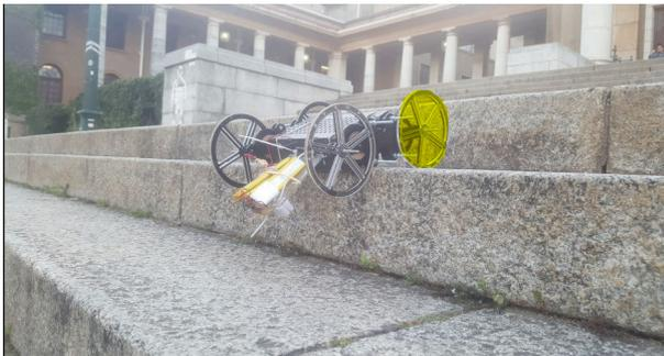
(e) step 5 of the desired motion for rotating the rear wheel on to the obstacle
