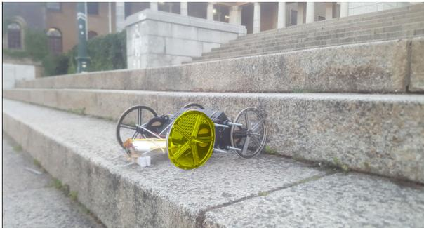
(a) step 1 of the desired motion for rotating the rear wheel on to the obstacle
