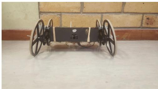
(a) Wheels buckling under the weight of the body
