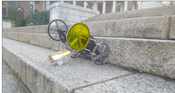
(b) step 2 of the desired motion for rotating the rear wheel on to the obstacle
