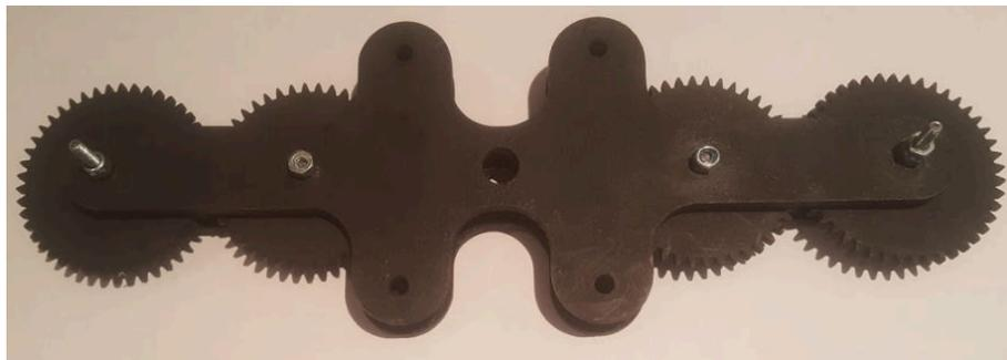
Figure 6.11: LIM version 1.0 fabricated from wood and assembled
