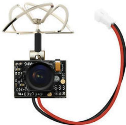
(a) Eachine TX01 camera, transmitter and RHCP antenna
